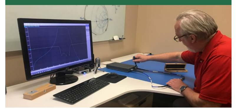
M Series VNAs deliver metrology-grade performance in a more economical package that excludes a number of advanced features: Vector Mixer Calibration, TRL Calibration, Frequency Offset, Time Domain, and Gating. These Vector Network Analyzers are small, can be powered by battery, and are ideal for use in laboratory and production testing in a variety of applications including filter tuning, antenna test and characterization, amplifier testing, etc.
