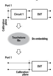
Allows users to mathematically exclude from the measurement result the effect of the fixture circuit connected between the calibration plane and a DUT. This circuit should be described by an S-parameter matrix in a Touchstone file.
