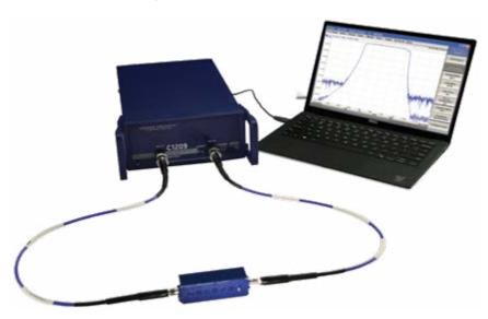
Cobalt 20 GHz VNAs have 135 dB dynamic range at 1 Hz IFBW, which allows them to maintain a wide measurement range at high measurement speeds. Measurement of all S-parameters of a BTS filter with full two-port and 801 measurement points with 1 MHz IFBW takes only 17.5ms while maintaining a measurement range of over 85 dB. This time is almost completely determined by the IFBW of the VNA. This measurement speed allows for real time tuning of high isolation BTS filters.
