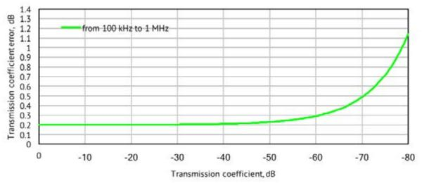
Specifications are based on matched DUT, and IF bandwidth of 1 Hz  $\,$
