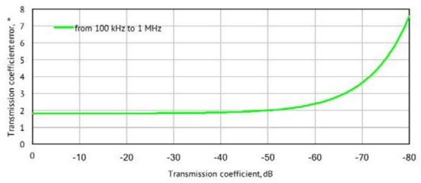
Specifications are based on matched DUT, and IF bandwidth of 1  $\rm Hz$
