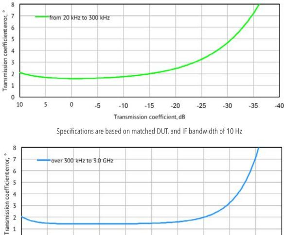
Transmission coefficient, dB Specifications are based on matched DUT, and IF bandwidth of 10 Hz
