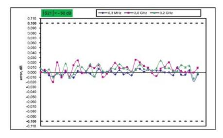
Low trace noise allows for particularly high-precision measurements. This graph shows the variation of the absolute value of the measurement error of  $S_{21}$  and  $S_{12}$  with a value of  $|S_{21}|$  and  $|S_{12}|$  -50 dB, using 42 different instruments. With the model's specifed accuracy of  $\pm$  0.1 dB, the trace clearly shows that the variations within the instrument pool is well below that figure. This confirms the precision of the instrument.
