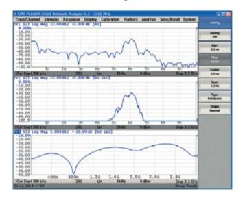
This function mathematically removes unwanted responses in the time domain, which allows the user to obtain a frequency response without effects of fixture elements.
