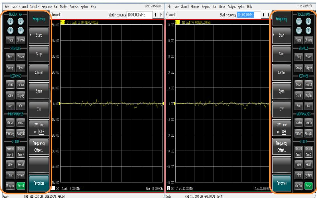
The favorite shortcut soft keys can be put together to simplify the operation for The soft panel can be put on left or right side of the screen. Or it can be hidden for operation convenience.
