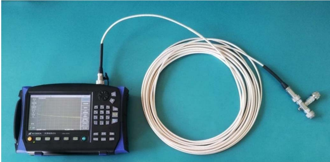
Cable loss measurement
