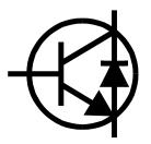
between the collector and the emitter so that they are normally reverse biased.
