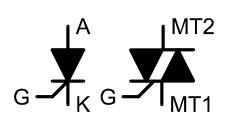
Thyristor terminals are the anode, cathode and the gate. The pinout of the thyristor under test will be displayed on the next press of the **scroll-off** button.
