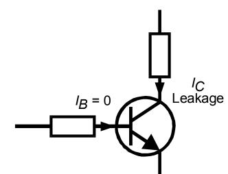
Leakage current Ic=0.170mA Older Germanium types however can suffer from significant collector leakage current, particular at high temperatures (leakage current can be <u>very</u> temperature dependant).
