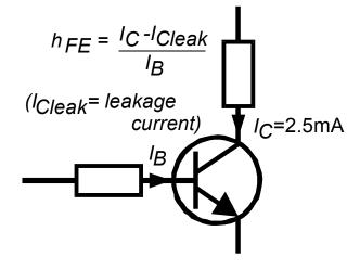
The gain of all transistors can vary considerably with collector current, collector voltage and also temperature. The displayed value for gain therefore may not represent the gain experienced at other collector currents and voltages. This is particularly true for large devices.
