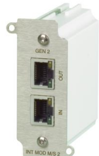
fig 7 - 10 Master Slave interface M/S-2. Note: the M/S-2 can only be used in SM15K
