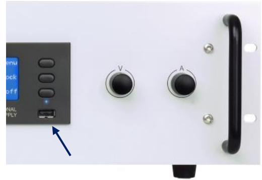
fig 5 - 7 The location of the front USB-connector.
