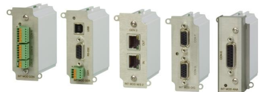
fig 4 - 8 Different interface modules can be plugged in.
