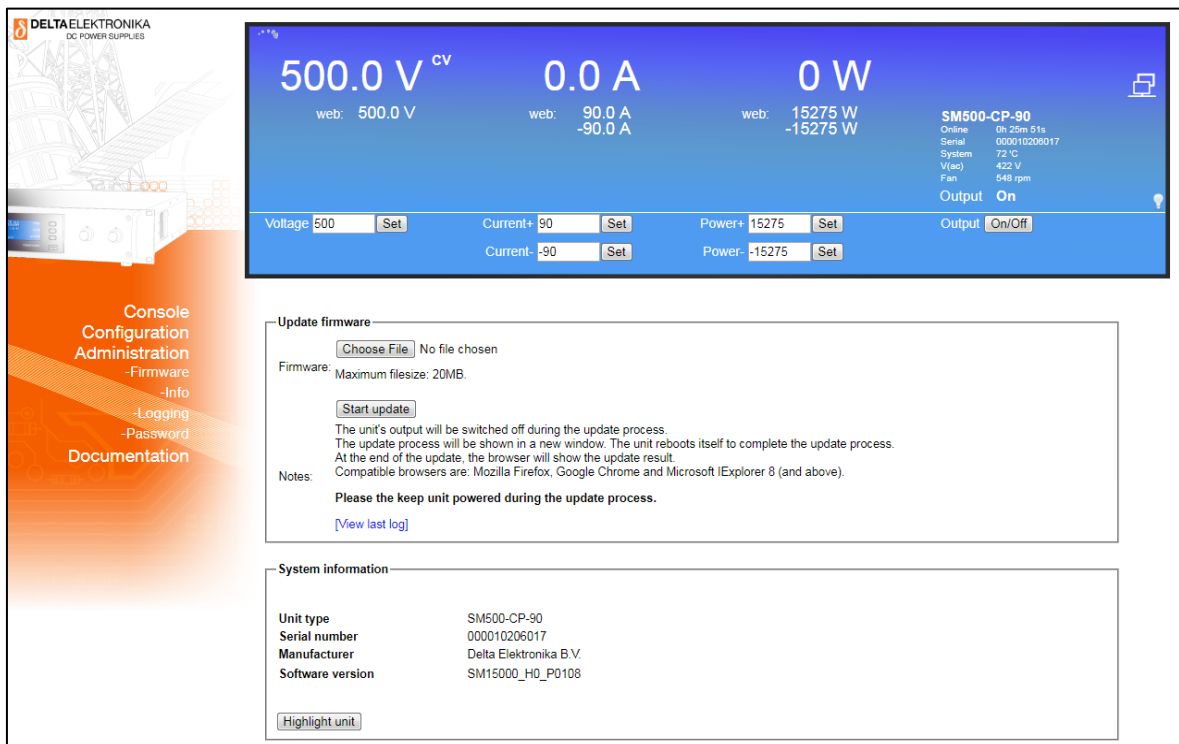
fig 6 - 3 - Via the web interface the downloaded firmware package can be uploaded to the unit.
