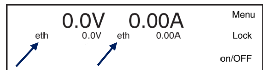
fig 5 - 18 The programming source appears before the settings. In this example both CV and CC settings are controlled via Ethernet.
