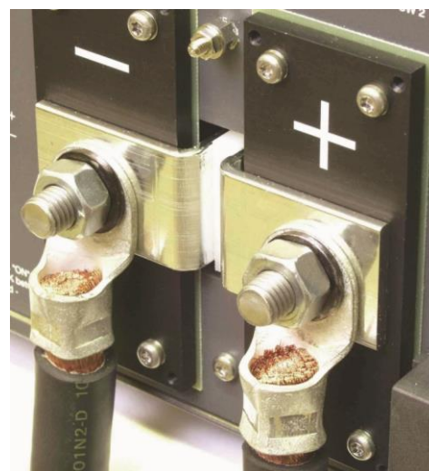
fig 4 - 1 Low resistive cable connection by mounting the cables directly on the DC output strips.
