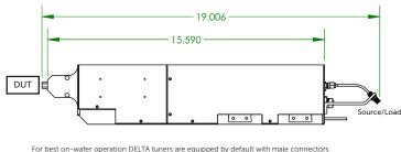
For best on-wafer operation DELTA tuners are equipped by default with male connectors DUT-side and female connectors Source/Load side. Different Configurations are possible on specific customer requests
