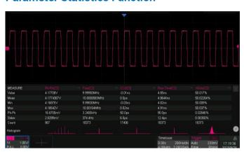
Statistics show the current value, maximum value, minimum value, standard deviation, and mean value of up to 12 parameters simultaneously. A histogram is available to show the probability distribution of a parameter. Trend and Track are available to show the parameter value vs. time.
