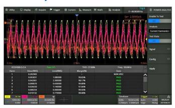
The Power Analysis option provides a full suite of power measurements and analysis, which greatly improve the measurement efficiency in switching power supplies and power devices design.
