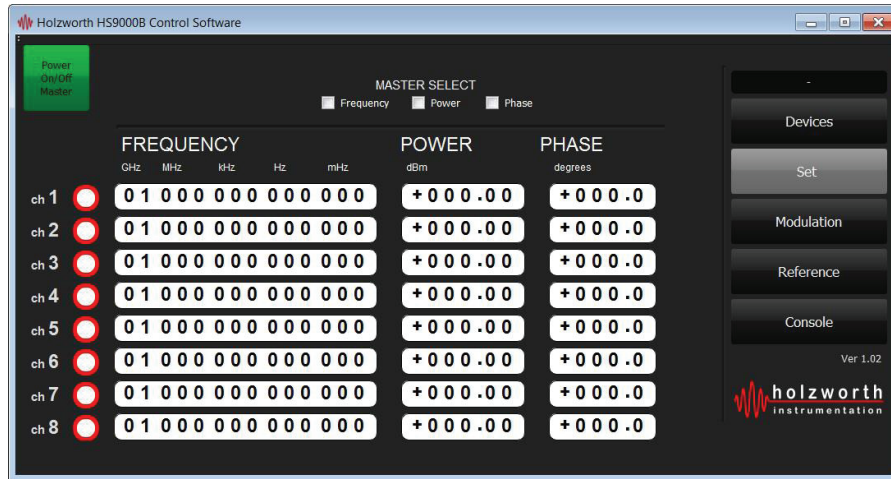
HS9000B SERIES MAIN CONTROL WINDOW
