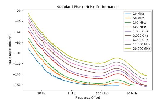
**40 GHz OPT-ULN PHASE NOISE PERFORMANCE** (*P*<sub>out</sub> = +10 dBm)
