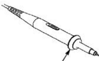
Figure 3-8: Finger Safety Ring of the Probe
