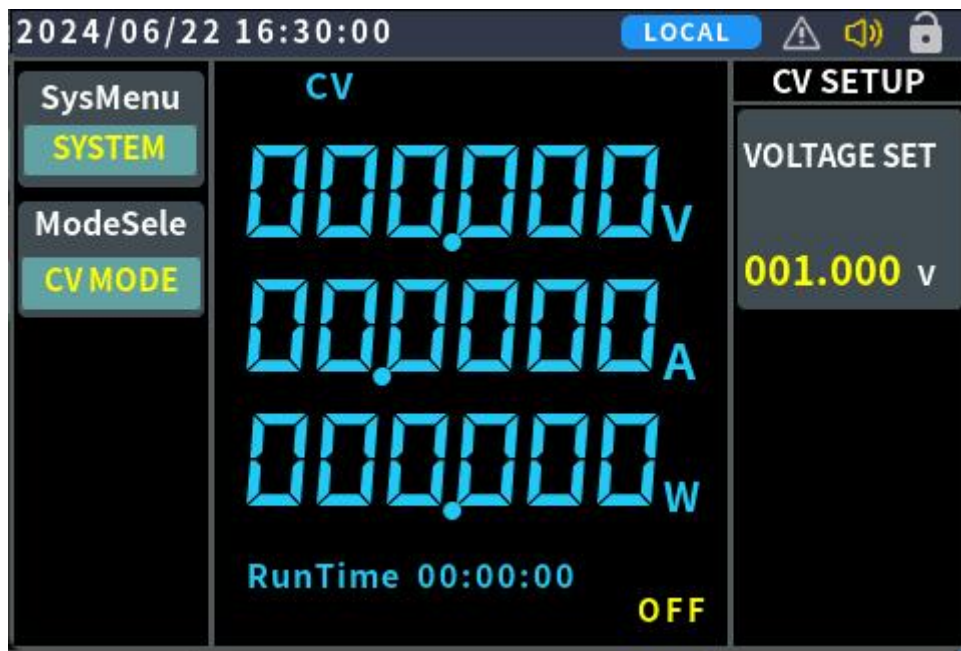
Figure 4.3.2-2 CV mode operation interface
