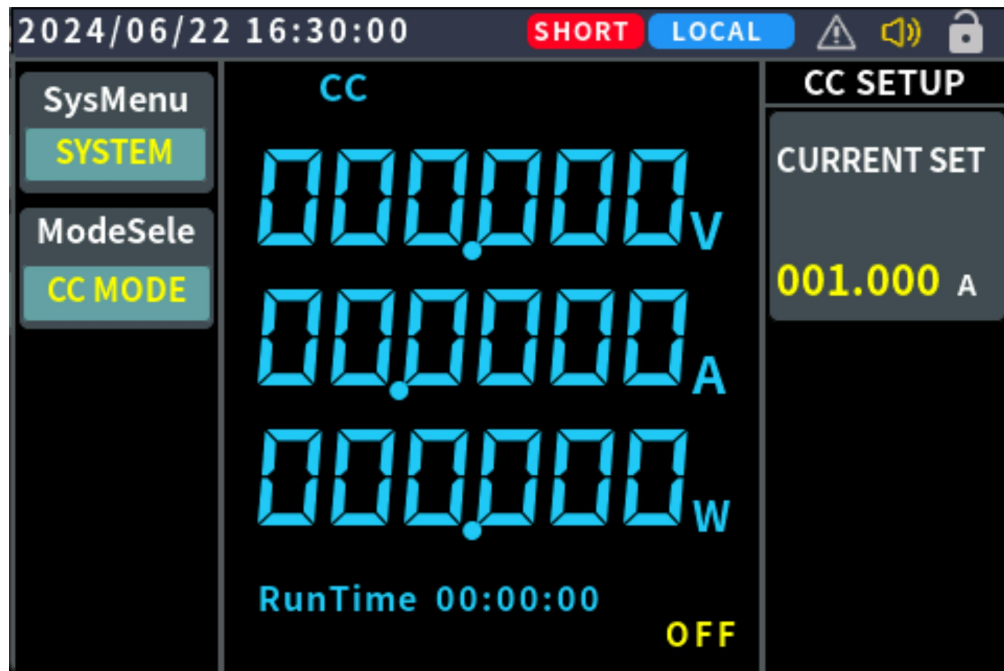
Figure 4.6-1 Short circuit simulation interface
