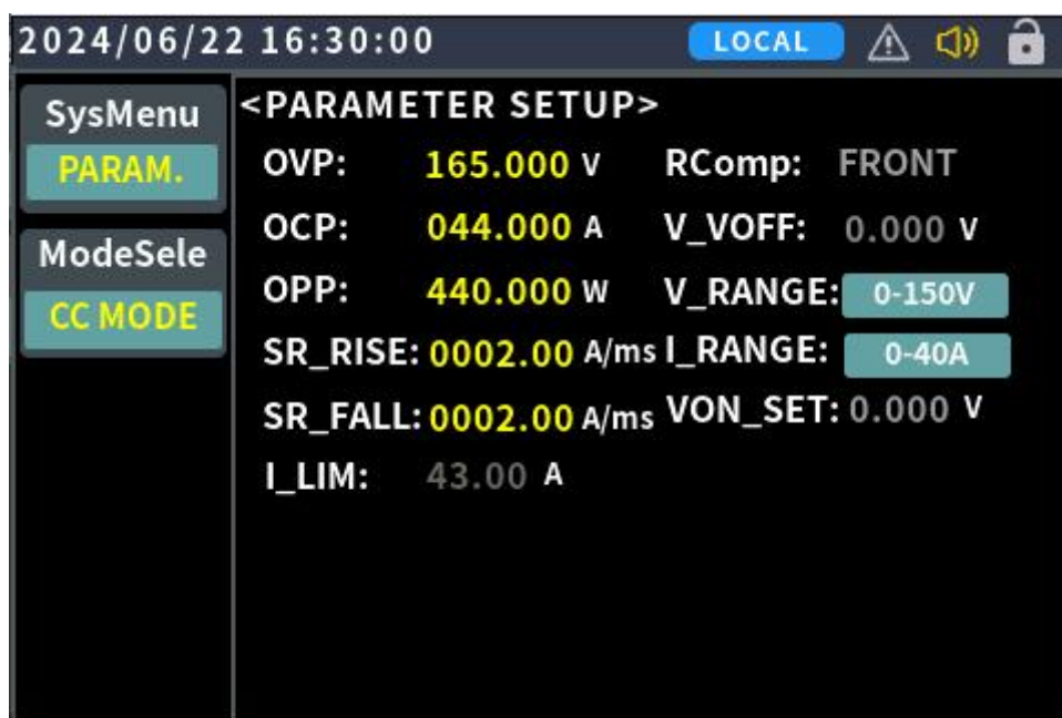
Figure 4-7-2 parameters setup page
