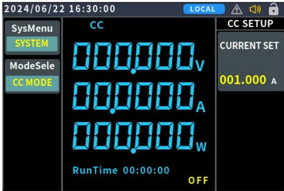
Figure 4.3.1-2 CC mode operation interface
