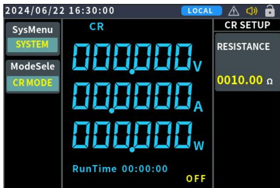
Figure 4.3.3-2 CR mode operation interface
