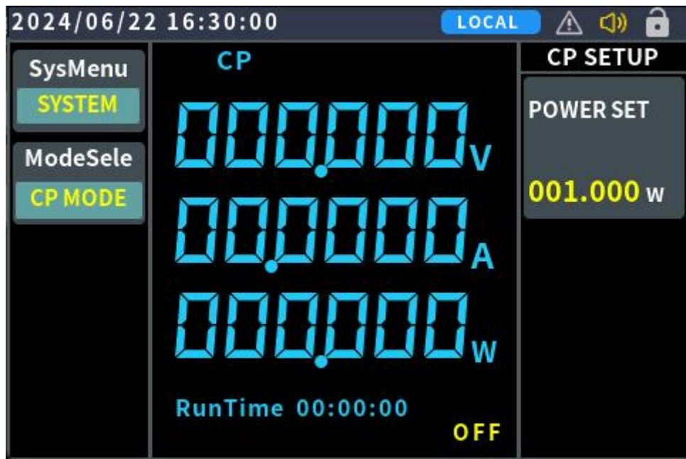
Figure 4.3.4-2 CP mode operation interface
