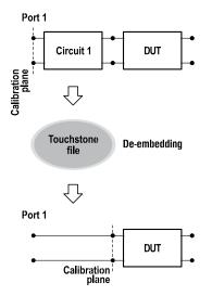
This function allows users to mathematically exclude from the measurement result the effect of the fixture circuit connected between the calibration plane and the DUT. This circuit should be described by an S-parameter matrix in a Touchstone file.
