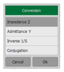
The function allows conversion of the measured S-parameters to the following parameters: reflection impedance and admittance, inverse S-parameters and conjugation.
