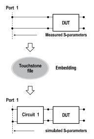
This function allows the user to mathematically simulate the DUT parameters after virtual integration of a fixture circuit between the calibration plane and the DUT. This circuit can be described by an S-parameter matrix in a Touchstone file.
