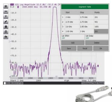
1-port VNAs (cable and antenna analyzers) have a large frequency range with the option of frequency scan segmentation. Among other benefits, this allows the user an opportunity to use the VNA, to realize the maximum dynamic range while maintaining high measurement speed.
