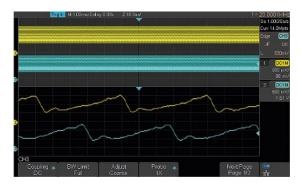
Using hardware-based Zoom technologies and max record length of up to 28 Mpts, users are able to over-sample to capture longer time periods at higher resolution and use the zoom feature to see more details within each signal.
