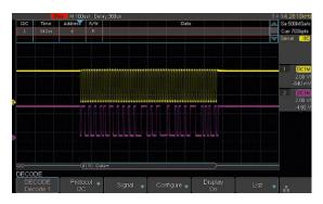
T3DS01000 displays the decoding through the events list. Bus protocol information can be quickly and intuitively displayed in a tabular format.
