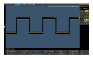
The T3DS01000 utilizes a hardware-based Pass/Fail function, performing up to 40,000 Pass/Fail decisions each second. Easily generate user defined test templates provide trace mask comparison making it suitable for long-term signal monitoring or automated production line testing.
