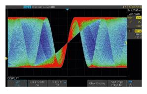
The color temperature display is similar to the intensity-graded trace function, but the trace occurrence is represented by different colors (color "temperature") as opposed to changes in the intensity of one color. Red colors represents the more frequent events, while blue is used to mark points that occur lest frequently.
