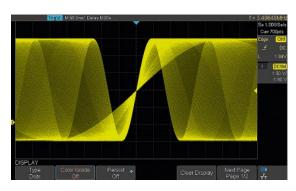
New display technology provides for fast refresh rates. The resulting intensity-graded trace is brighter for events that occur with more frequency and dims when the events occur with less frequency.
