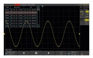
Playback the latest triggered events using the history function. Segmented memory collection will store trigger events into multiple (Up to 80,000) memory segments, each segment will store triggered waveforms and timestamp each frame.
