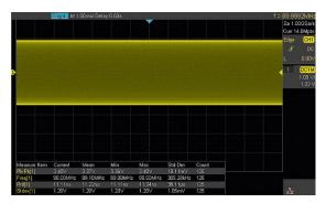
At any one timebase, T3DS01000 can measure using all acquired sample points. This ensures the accuracy of measurements while the math coprocessor decreases measurement time and increases ease-of-use
